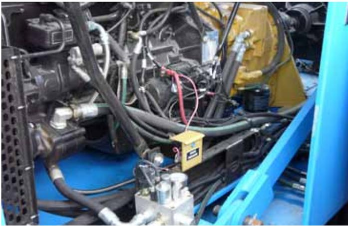
Eaton's Aeroquip MatchMate Plus hose and fittings are strung from head to toe on the Lampson mega crane.
