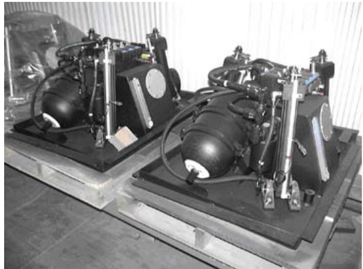
Eaton designed motion bases for the SimEx-Iwerks TurboRide feature vane pumps, cylinders, valves, manifolds, hoses, and fittings from Eaton's Hydraulics Group.
