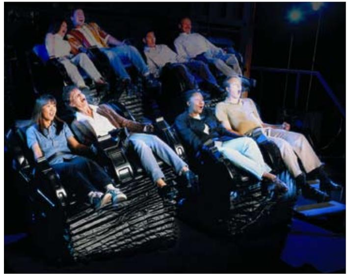
SimEx-Iwerks' largest project to date includes 75 TurboRide two-seat modules, each equipped with an Eaton motion base. The units are individually controlled for gentle to vigorous motion.
