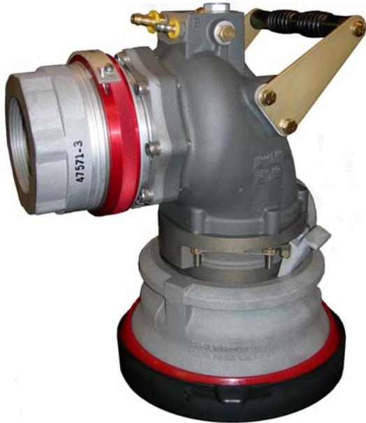
The Check Valve, previously located under the Fuel Sense fitting, is now part of the Closing Time adjustment and is no longer subject to damage from over tightening of the fitting. To improve the maintainability of the Coupler, the outlet adapter is now replaceable and no longer part of the cast housing. Carter has also provided for an outlet fitting on the Control Elbow that can be used to attach a Hydrant Valve deadman command line.
