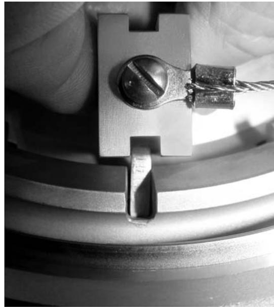
Refer to the photo, above, and check each lug separately by placing the lug part of the gauge onto a lug. If the gauge sits squarely onto the I.D. of the coupler with the tip of the lug not touching the bottom of the gauge slot, the lug or the actuating collar has excessive wear. Inspect all 16 lugs. A lug in good condition will raise the gauge away from the coupler I.D. allowing it to rock on the lug.
