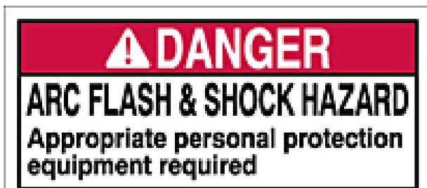
Fig. 1. Example of an Arc-Flash Hazard Warning label per NEC [2], Section 110.16
