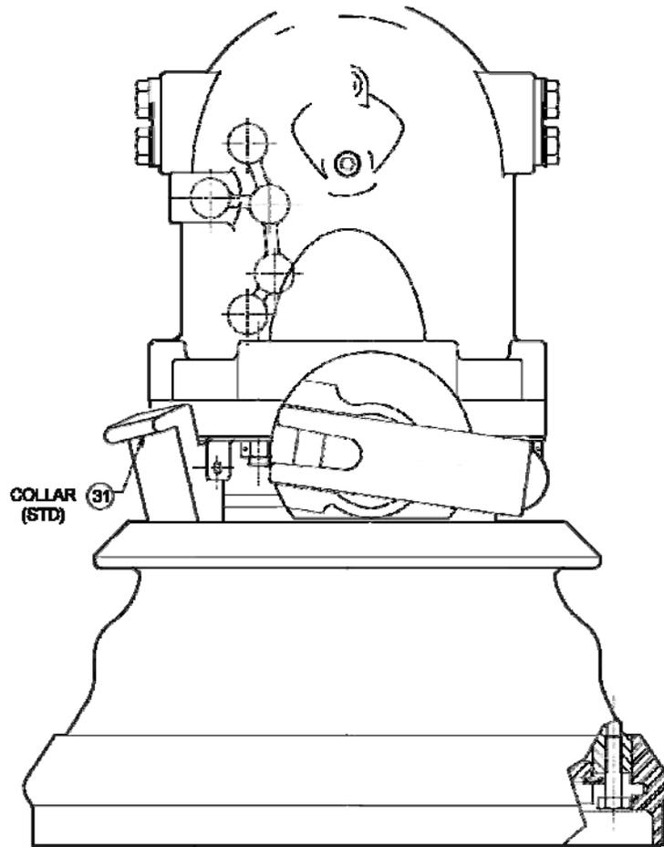
The Collar Lock Assembly is assembled to the coupler in location shown using two of the studs from the elbow assembly and the existing Nuts (3-3) and Washers (3-2).
