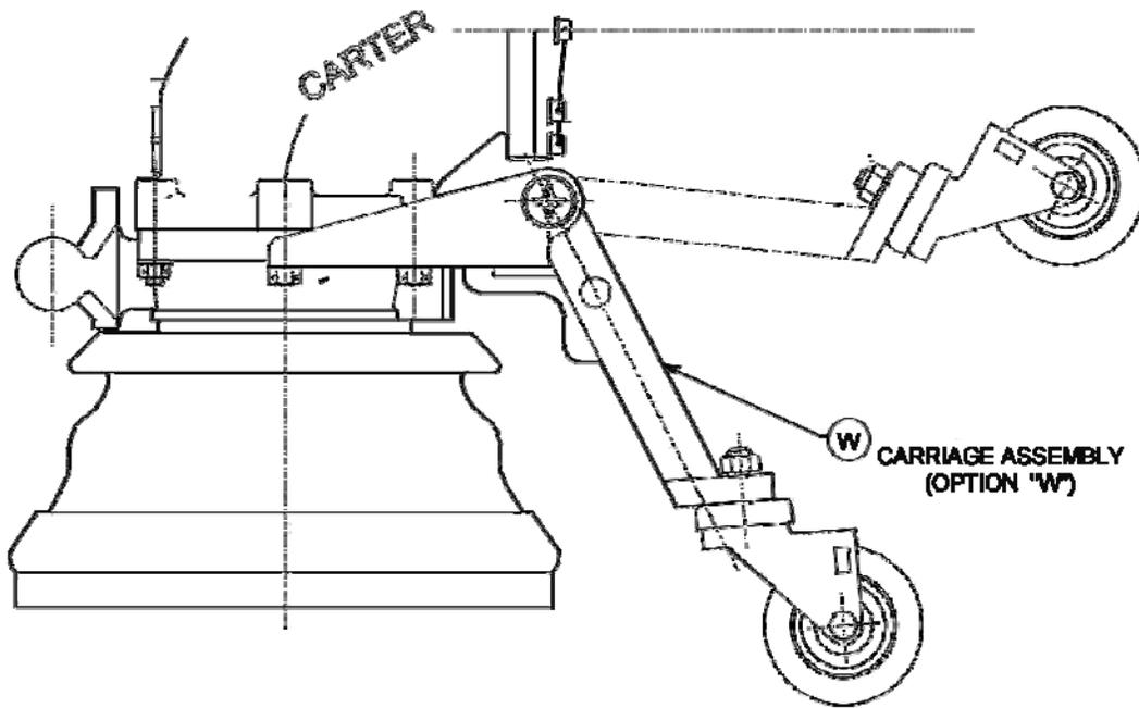
The carriage is assembled by removing four (4) of the Nuts (3-3) and Washers (3-2), placing the carriage in place and reinstalling the nuts and washers as noted in paragraph 11.9.D.
