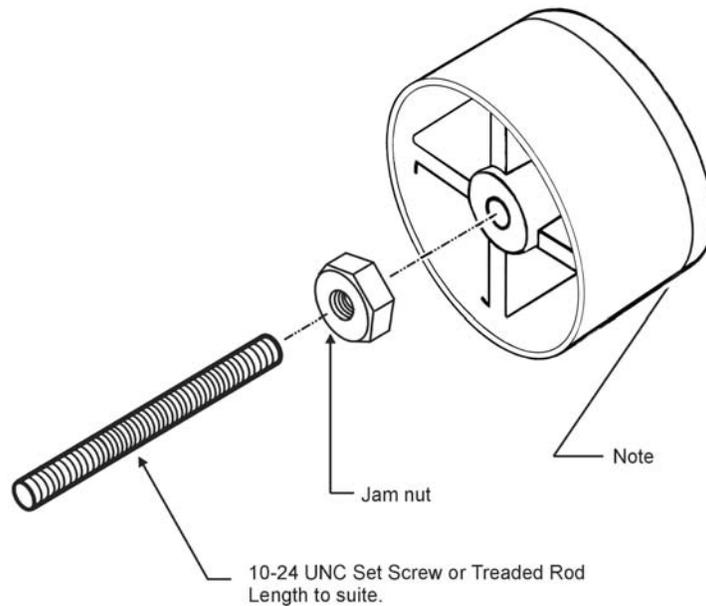
**Note:** Install set screw into (2) Outer Piston (23889) and fix with the jam nut. Using a hand drill fixed in a vise rotate the assembled tool at maximum speed of the drill. Using a long strip of emery cloth chamfer the edge of the piston (edge opposite the knife edge) to allow for ease of installation into regulator for lapping. See paragraph 8.2 for lapping instructions.
