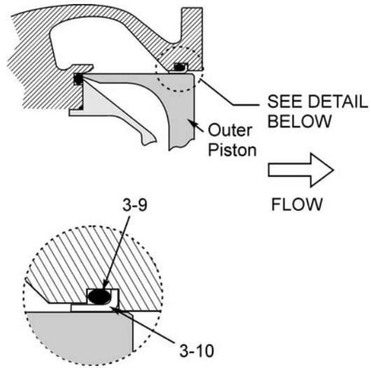
Outer Piston Seal Installation
