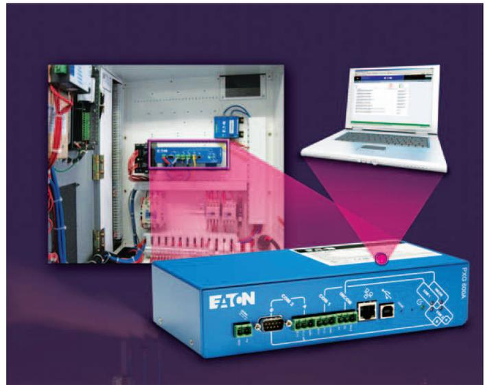
*"The data provided by the gateway will be used by the building automation system to determine how the facility can save energy. The company is also using data from the gateway to compare its actual usage against actual billing from the utility."*
