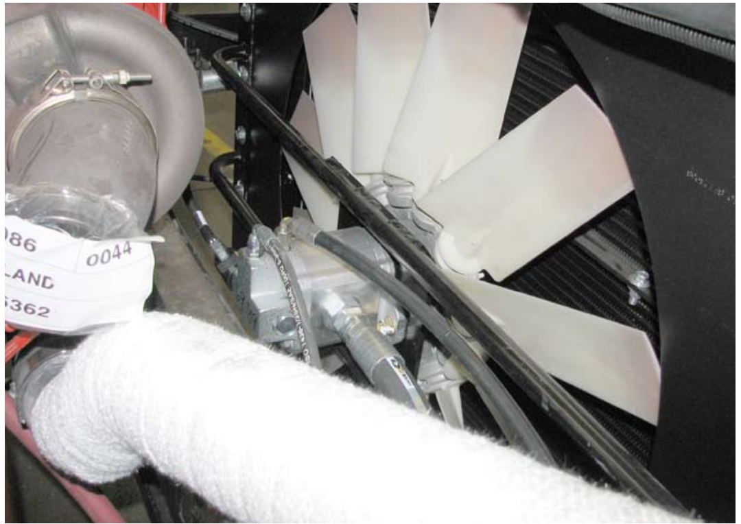
Eaton gear motor (mounted to cooling fan) with special electronic control proportional relief in motor's rear cover.
