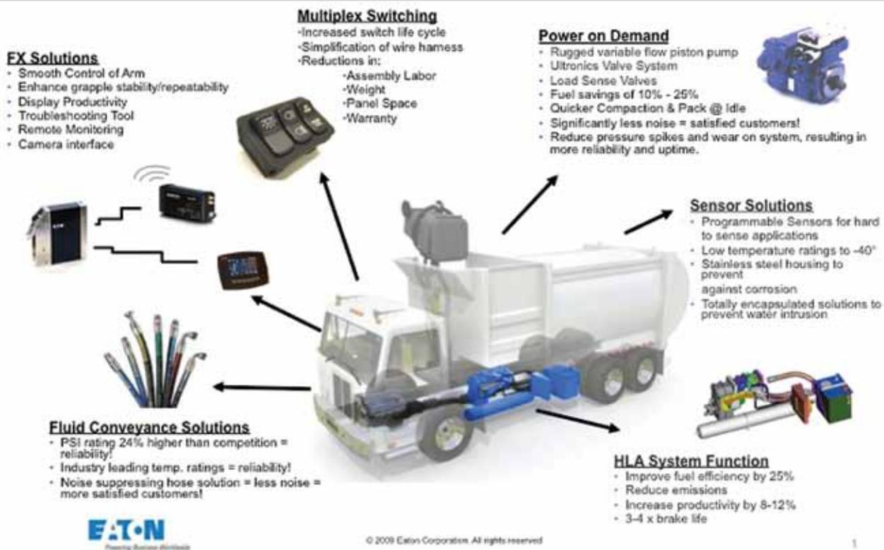
Eaton's Aeroquip® GH493 half-bend radius, high-pressure hose assembly that withstands tight bend radii required on the refuse truck.
