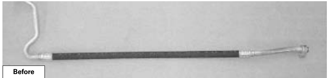
Figure 1. Failed Hose Assembly. Note crimp fittings.
