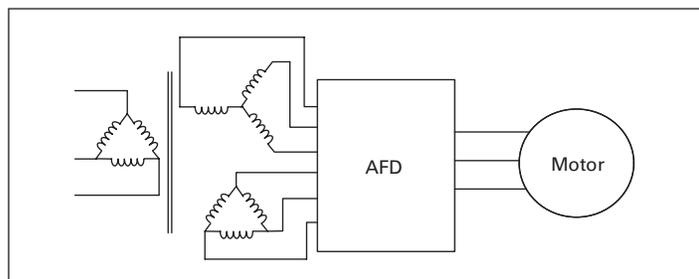
**Figure 4. 12-Pulse Converter**
