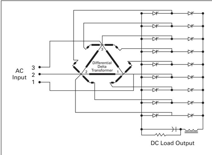
**Figure 8. Clean Power (18-Pulse Converter)**
