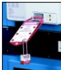
All breakers can be padlocked to secure the breaker in all three positions. An optional key interlock (not shown) can also secure the breaker in each position.
