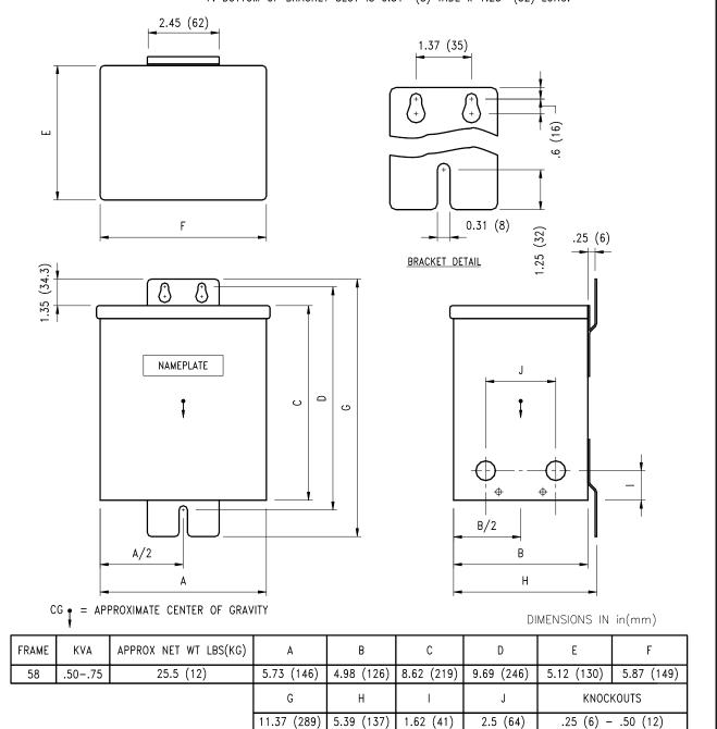
THIS DIMENSION DRAWING IS FOR REFERENCE ONLY. IT IS NOT TO BE REGARDED AS INDICATING THE EXACT DETAILS OF CONSTRUCTION.
