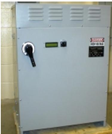
Figure 3: Cutler-Hammer's Sag Ride Through device, available in ratings from 20 kVa to 700 kVa, responds to sags in only 1/8 of a cycle to correct input voltages ranging from ten to seventy percent reduction in RMS voltage.
