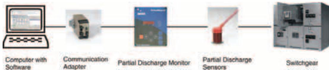
A complete partial discharge monitor system consists of four major components:
