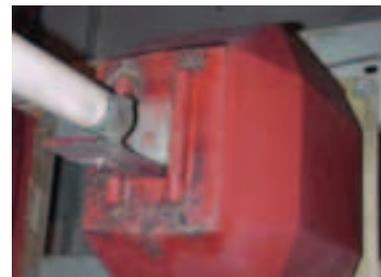
*Insulation Damage on Voltage Transformer*
