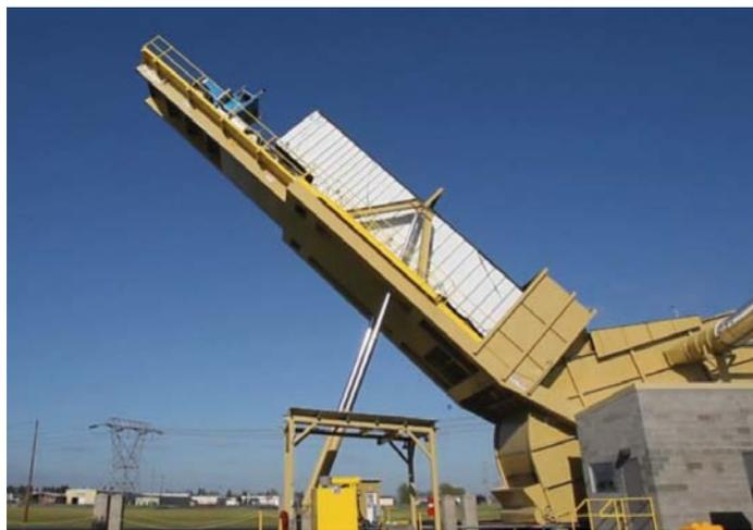
Biomass enters the system via a "truck dump" that tips a tractor-trailer rig on end to empty wood slash into a hopper. (Photo courtesy of *The Register-Guard*)
