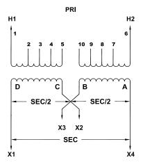
DFTR DATE Cutler-Hammer THE INFORMATION ON THIS DOCUMENT IS CREATED BY CUTLER—HAMMER. IT IS DISCLOSED IN CONFIDENCE AND IS ONLY TO BE USED FOR THE PURPOSE IN WHICH IT IS SUPPLIED. Juarez, Mexico A. CISNEROS 2/16/05 TITLE DRY TYPE TRANSFORMER WIRING SCHEMATIC DATE 2/16/05 APPD C.ROMO S.0. TYPE TRANSFORMER REVISION DWG SIZE SHEET 01 OF 01 FEDERAL ID NO PRODUCT CODE G.O. DWG 0.1**TRANSFORMERS**
