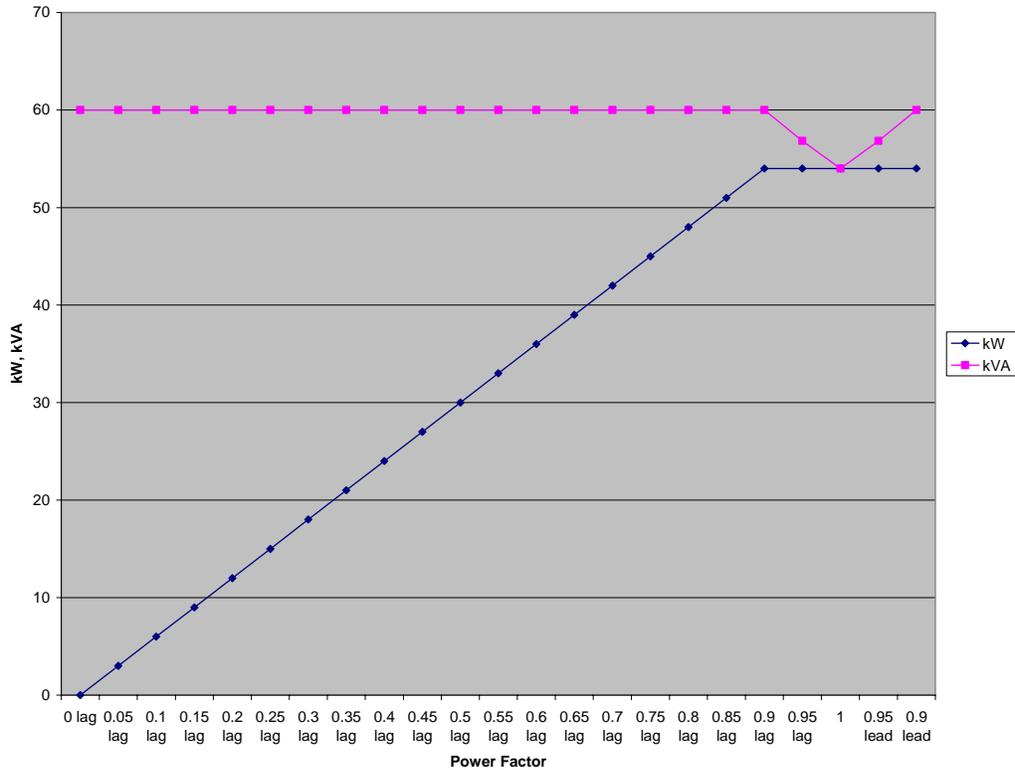
**Figure 1. Comparison of kW and kVA limits for a 60 kVA, .9 pf UPS**
