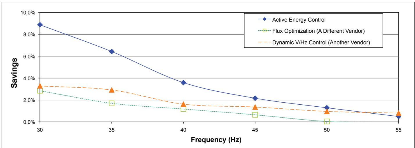
Figure 4. Energy Savings for Various Dynamic V/Hz Modes (Compared with Linear Mode)
