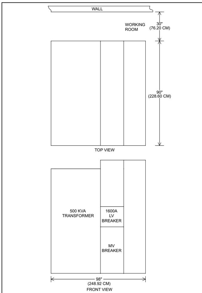
**Figure 8. Integrated Unit Substation (IUS).**
