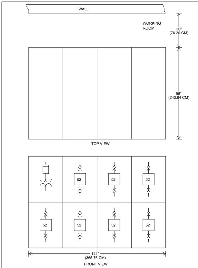
**Figure 5. Standard Metal-Clad Switchgear.**
