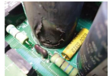
Photo 2. Random component failure.
