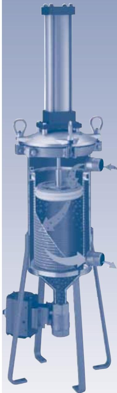
The DCF-800 filter has a patented cleaning disc that moves up and down the filtering screen, scraping debris from the screen and collecting it in a chamber at the bottom of the filter. Debris is periodically purged from the collection chamber by a discharge valve, in a process that takes less than seven-tenths of a second — with no interruption in production.
