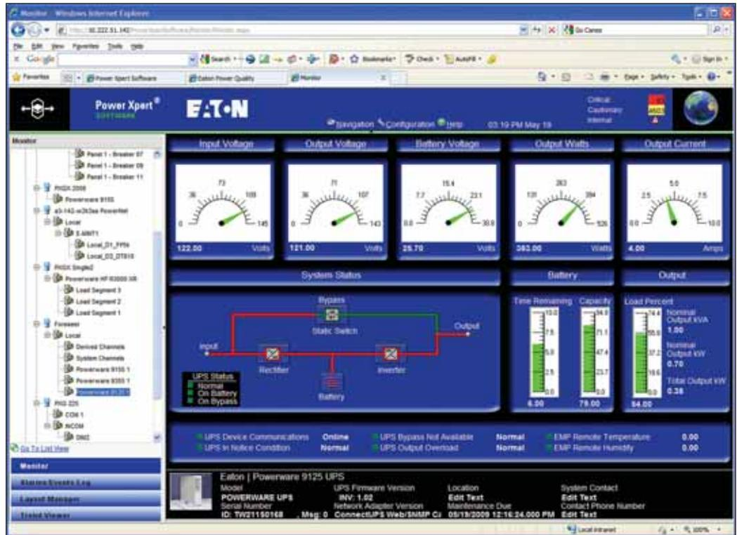
Graphic templates are built into the software for all standard Eaton devices. Viewing all of the most vital parameters along with self-explaining legends and one-line diagrams are available at a glance. Device-specific information is gathered at the bottom of the screen, including a product picture, location, system contact, maintenance schedule and asset serial number.
