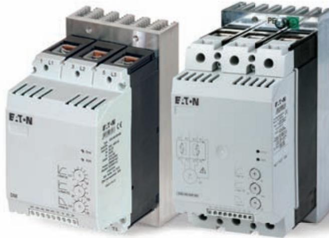
With a focus on small size and ease of installation, Eaton's DS6 line of reduced voltage solid-state soft start controllers is designed to meet your needs for reliable and efficient soft starting. Designed to control the acceleration and deceleration of three-phase motors, the DS6 Series is available for current ranges from 40 to 180 amps.
