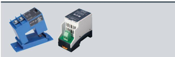
CurrentWatch™ products are perfect for providing improved reliability, predictive diagnostics, feedback and monitoring for all types of electrical equipment. Simply run a conductor wire through the sensing aperture, wire the outputs to your controller, and installation is complete. With features such as split-core housings that wrap around existing wires, industry-standard outputs and self-powered models available, sensing current has never been easier.
