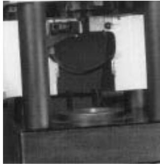
2. OPEN pusher halves and place T-410-25 adapter ring (ET4000AR-001).
