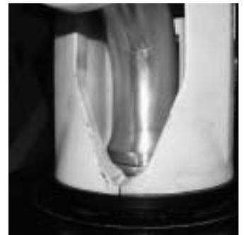
9. CLOSE the pusher halves and begin crimping by activating the pump with turning on the switch. When the pusher halves or spacer ring (if applicable) contacts the base adapter ring, the crimp is complete.
