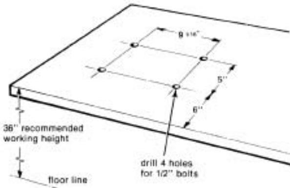
**Figure 2 - Lifting Hole Layout on ET4000 Press Top Plate**
