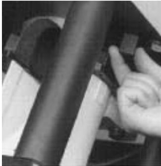
1. HOLD SWITCH "ON": As ram starts downward, rotate the ram return stops outward from their inward position. RELEASE SWITCH. Ram will return to the full upright position allowing enough clearance for insertion of required tooling.
