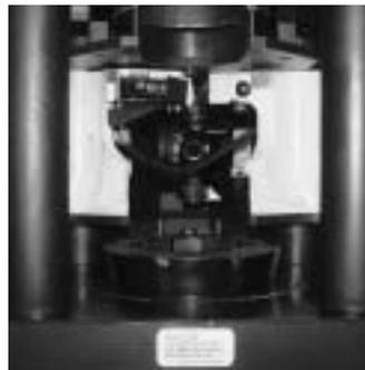
7. SELECT the proper collet assembly for hose type being crimped as referenced in the Crimp Specifications Manual and insert the collet assembly into the base adapter ring.
