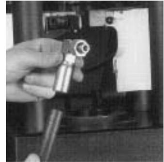
3. SELECT proper size collet (referenced in the Crimp Specifications Manual) for hose type and size being crimped. INSERT collet halves into adapter ring. PLACE proper size hose end on hose. Be sure to bottom the hose.
