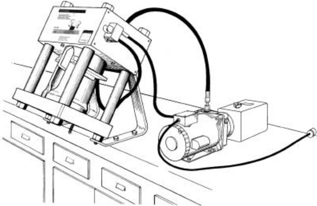
**CAUTION:** Throughout the Check-out Procedure, check hose assembly/adaptor connections for any leaks. TIGHTEN if necessary. For-Seal Swivel Nut Torque for hose assembly; 32-35 ft. lbs. Check oil lever in power unit. The oil reservoir was filled at the factory, however, if oil is required use ISO 32 (SAE 10W).
