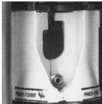
5. CLOSE pusher halves. HOLD SWITCH ON. When spacer ring (shown here in black) bottoms on adapter ring below it, the crimp is complete.
