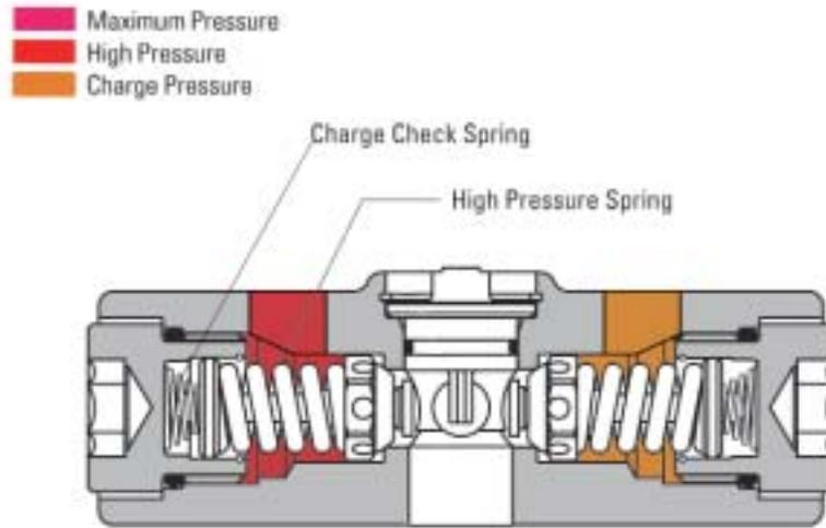
**Figure 5 – High Pressure Relief Valve - Normal Operations**
