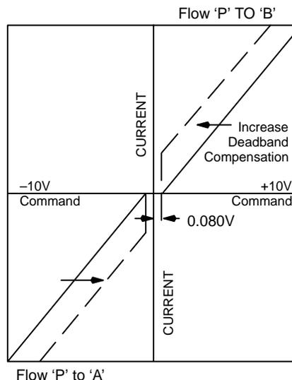
Figure 8. Amplifier Current Gain
