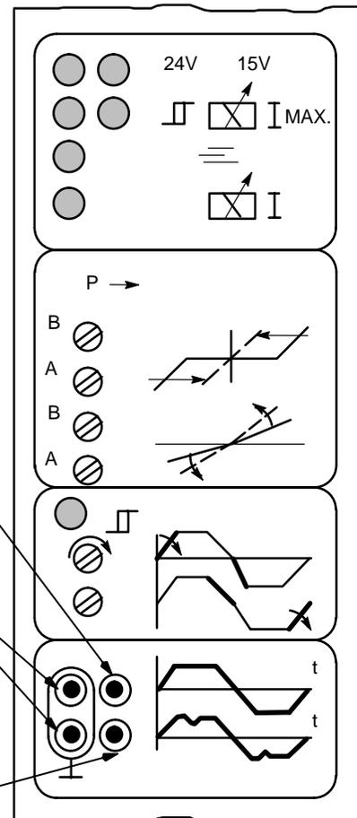
Figure 13. Proportional Valve Amplifier Set-Up Procedure
