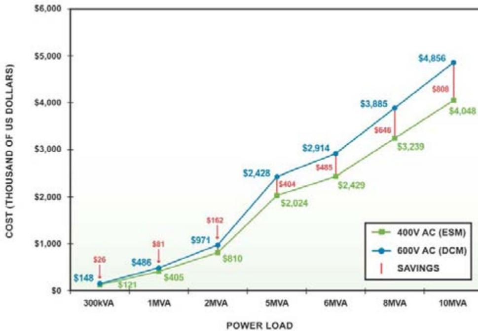
Chart 8: First-year OPEX (400V AC Energy Saver Mode vs. 600V AC double conversion mode)
