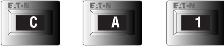
Figure 1: Clutch Abuse Indication
