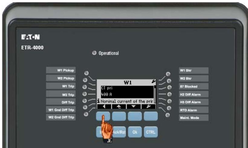
The CT pri (primary external CT settings), CT sec (secondary external CT settings), and XCT (ground / neutral CT settings) should all be set using similar steps. When all the CT settings have been selected and saved, select the soft key under the left arrow to return to the "System Para" level.
