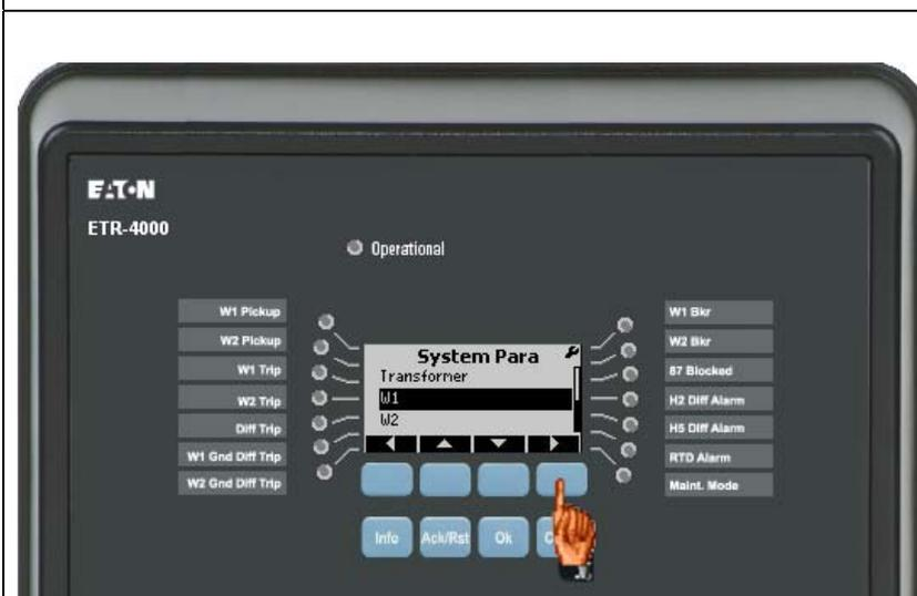
Select the desired Phase Sequence parameter setting using the soft keys under the up and down arrows. Press the soft key under “Ok”. Save the selected parameter (see Section 2 – Saving Parameters).
