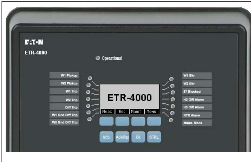
When the ETR-4000 is first powered up, the protective elements listed in Table 2 are enabled in each setting group.
