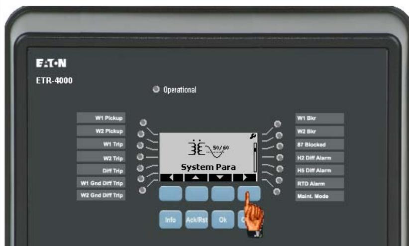
From the “System Para” screen, press the soft key under the right arrow to access the “System Para” menu.
