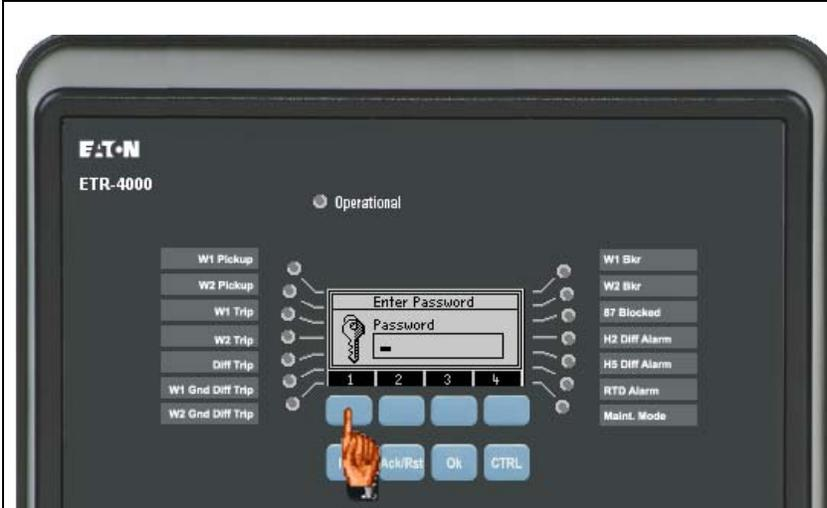
Enter the four-digit password as described in Section 1: Password Entry. After the password has been entered, press the “Ok” soft key.
