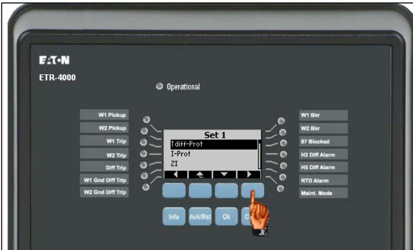
To program current protection, press the soft key under the right arrow while "Tdiff-Prot" is highlighted. This will display a list of current protection settings under "Tdiff-Prot."
