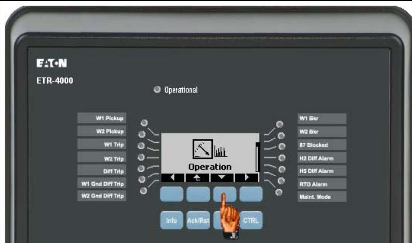
From within the “Operation” screen, press the soft key under the down arrow to access the next parameter screen “System Para” (System Parameters).
