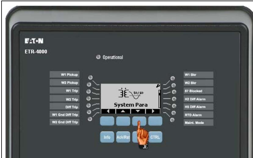
Select the soft key under the down arrow key to reach the “Protection Para” (Protection Parameter) screen.
