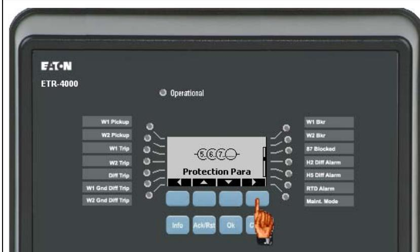
To set the protection parameters, use the soft key under the right arrow to enter the “Protection Para” menu.
