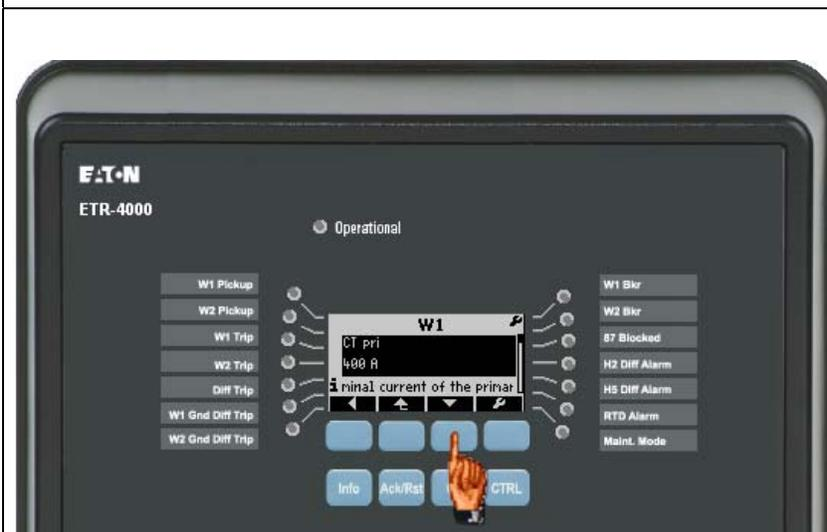
The User may change the frequency or, if the frequency is correct, use the soft keys under the up or down arrows to access additional system parameters.
