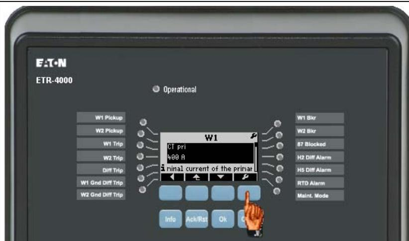
To edit any parameter, press the soft key under the wrench icon. To edit parameters, the User must enter a valid password (see Section 1: Password Entry).
