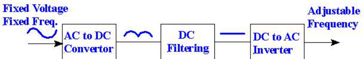
FIGURE 3 - Typical Variable Frequency Drive Hardware Configuration
