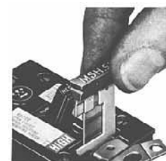
Heater Element Installation
