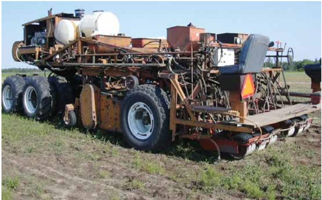
*Carrots are being planted at record speeds with a Vogel seed planter that has been retrofitted with EATON's EFX controller and CONTROL F(x) software.*
