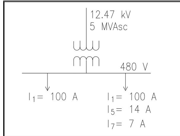
**Figure 3.** Example Power System with Linear and Harmonic Loads
