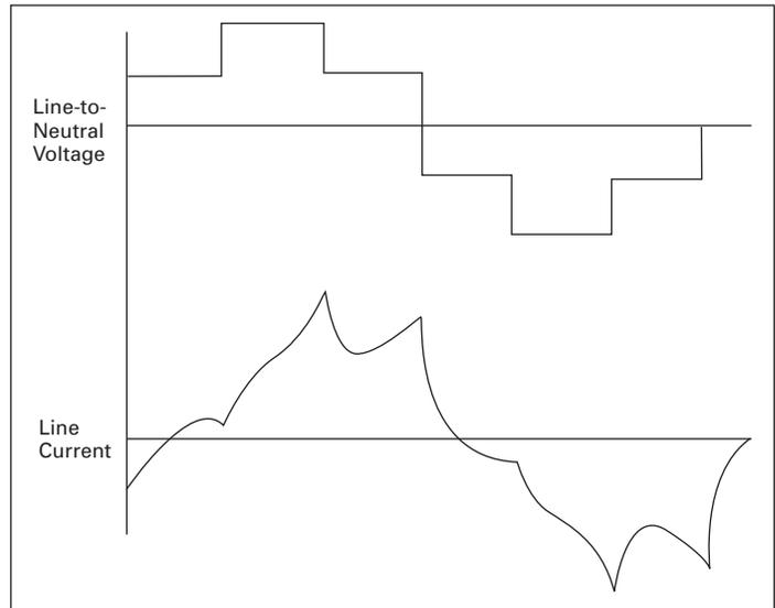
**FIGURE 2. TYPICAL VVI VOLTAGE AND CURRENT WAVEFORMS**
