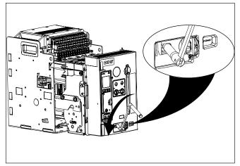
Step 3: Carefully push the circuit breaker into its compartment until it stops. The extension rails can now be folded up and latched.
