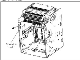
Step 2: Lower both rails down into their extended and locked position.
