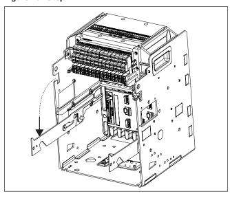
Step 3: Carefully place the circuit breaker on the extended rails. Be certain that the circuit breaker's metallic support wheels (two on each side of the circuit breaker) are properly seated on the extension rails. With breaker properly seated on the extension rails, slide the breaker fully into the cassette and raise both rails up into the cassette so that they engage the extension rail latch. The breaker is now in the cassette in the DISCONNECT position.
