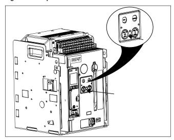
Optional electrically operated accessories are available to automatically close/trip a manually operated breaker.
