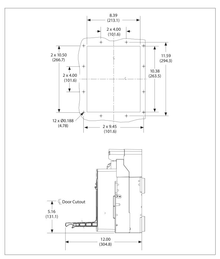
Figure 56. Three-pole fixed breaker - front view door cutout detail dimensions in inches (mm).
