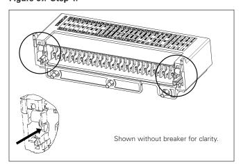
Step 2: (Drawout breakers) Once both latches are released the inner cradle can be compressed until the tool slot is visible. Insert a screwdriver vertically into the slot to hold the inner cradle in place and improve arc chute access.
