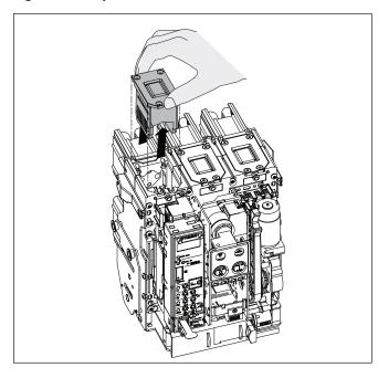
Step 5: Follow the same procedure to remove the remaining two arc chutes.
