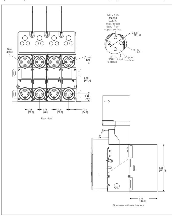
Figure 58. Four-pole fixed breaker overall views and dimensions in inches (mm) (UL 800-1200 A/IEC 630-1600 A).
