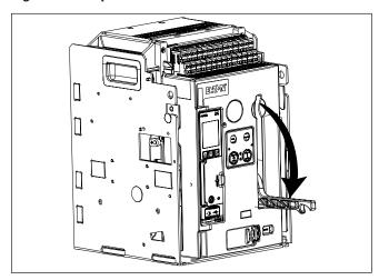
Step 3: Standard manually operated circuit breakers are closed and opened by hand using the Manual ON and Manual OFF buttons located on the front of the circuit breaker. To perform either operation, press and release the appropriate button. The status of the contacts (open or close) is indicated in the Contact Status Window just above the pushbuttons on the front of the breaker.
