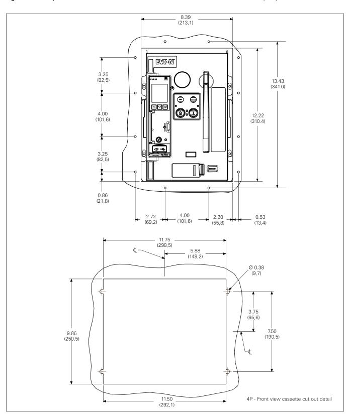
Figure 45. Four-pole drawout cassette - front view door and cassette cutout details in inches (mm).
