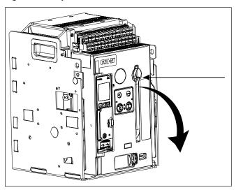
Step 2: It takes approximately seven full downward strokes to complete the charging process. It is possible to manually recharge the spring immediately after closing the breaker, before it has been tripped open. The status of the spring (charged or discharged) is indicated in the mechanism spring status window just above the pushbuttons.
