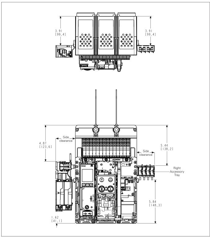
Note: A minimum of 2 in. (50.8 mm) of side clearance is required.
