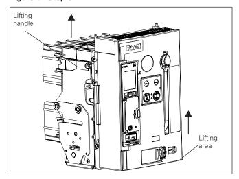
Step 4: Repeat Step 3 for a drawout cassette. The cassette is provided with a lifting indentation on each side.
