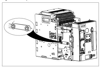
Keep in mind that all drawout circuit breakers are provided with safety interlocks to prevent inserting circuit breakers into incompatible drawout cassettes. Do not force a circuit breaker that does not roll smoothly into the casette.
