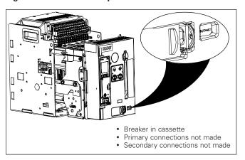
Figure 16. DISCONNECT position.
