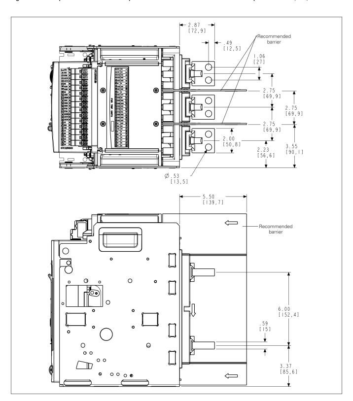
Figure 37. Three-pole drawout cassette - top/side views with horizontal universal bus adapters in inches (mm).
