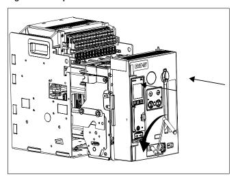
Step 4: The breaker is ready to be levered. With the circuit breaker OPEN, rotate the levering tool clockwise to and through the different available positions (DISCONNECT, TEST, CONNECT).
