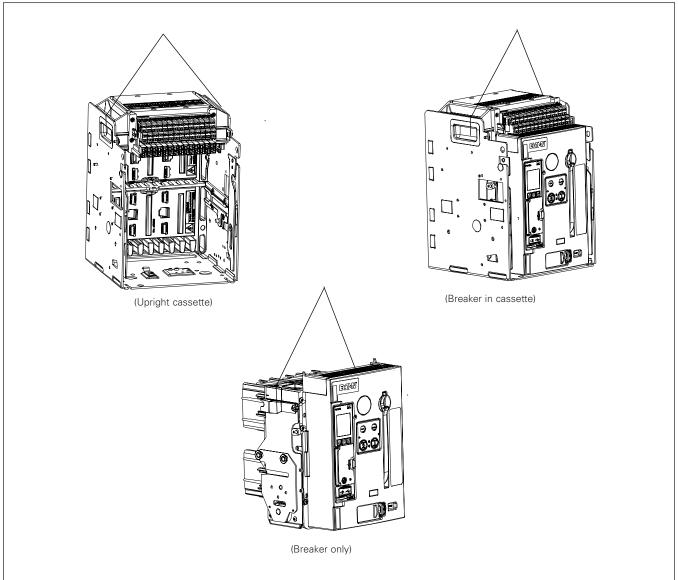
**Note:** When using an appropriate lifting device, attach the lifting harness in the locations shown in Figure 10 that best fits the circumstances.
