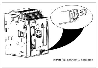
Step 5: To remove the circuit breaker from any position or from the compartment completely, reverse the insertion procedure just described in Steps 1 through 4 by rotating the levering tool in a counterclockwise direction. When the DISCONNECT position is reached, the circuit breaker will no longer move out of the cassette as a result of rotating the levering tool. At this point, the circuit breaker can be pulled out of the cassette onto its drawout rails.
