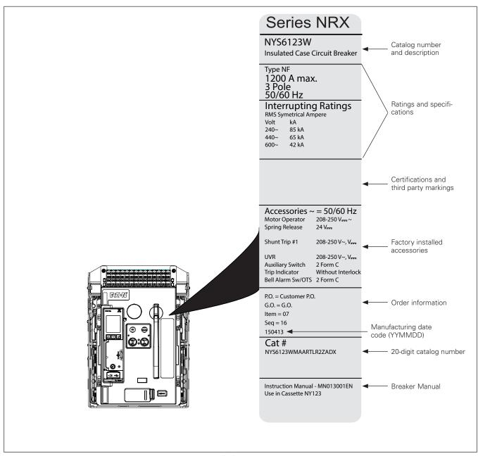
The circuit breaker configuration is fully described by a 20-digit catalog number located on the name plate. The drawout cassette can be identified by a 14-digit catalog number. An overview of the catalog number code can be found in the catalog at www.eaton.com/seriesnrx. Unique individual circuit breakers are identified by the older information: G.O. item, and sequence numbers. Taken together, these are equivalent to a serial number.
