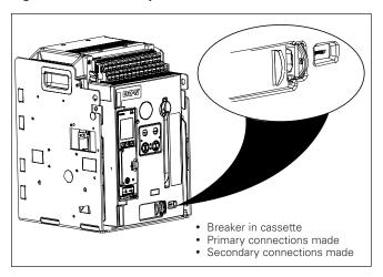
With the circuit breaker sitting solidly on the extension rails in its WITHDRAWN position, proceed with the following five steps to move the circuit breaker through its other positions
