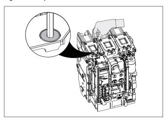
Step 4: Lift the arc chute up and out of the arc chamber.
