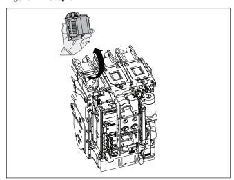
Step 7: When inspections are complete, secure arc chutes in place with their mounting screws. Remove the screw-driver and verify that the secondary contact assembly inner cradle re-latches.
