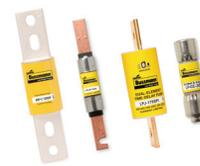
Motor inrush requires the selection of branch circuit overcurrent protective devices that will not open needlessly from normal high inrush currents. At the same time, overcurrent protective devices need to provide a high degree of branch-circuit, short-circuit, and ground-fault protection if a short circuit or a ground fault occurs in the motor branch circuit.
