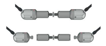
Tension links function as clamp fasteners until redundant initiators release their actuator shafts to facilitate separation in V-band (Marman) clamp applications.
