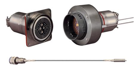
The pin puller depicted on the right end of the cable assembly facilitates electrical initiation for this umbilical connector. Mechanical redundancy is facilitated by the lanyard attached to the plug assembly.
