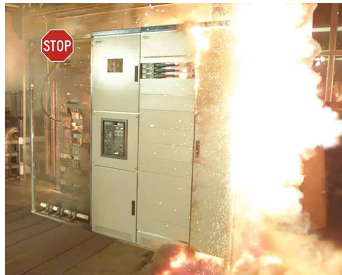
Figure 17. Development of temperature and pressure in a switchboard during internal arc
