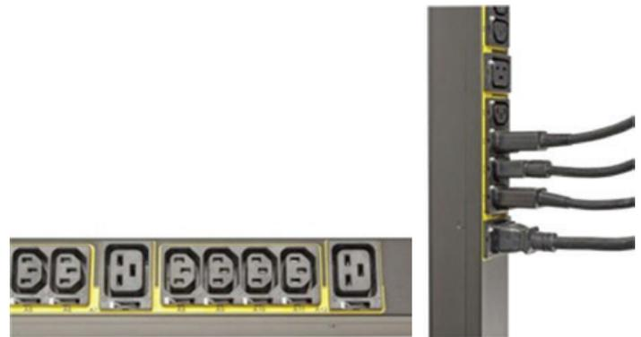
**Figure 3.** IEC outlet grips provide plug retention and eliminate the need for intrusive cable management that often blocks airflow and decreases serviceability.
