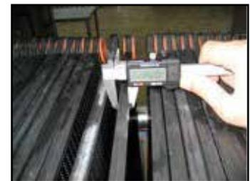
**Fig. 1:** Measuring the pressing edge
