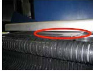
**Fig. 4:** Warped filter plate
