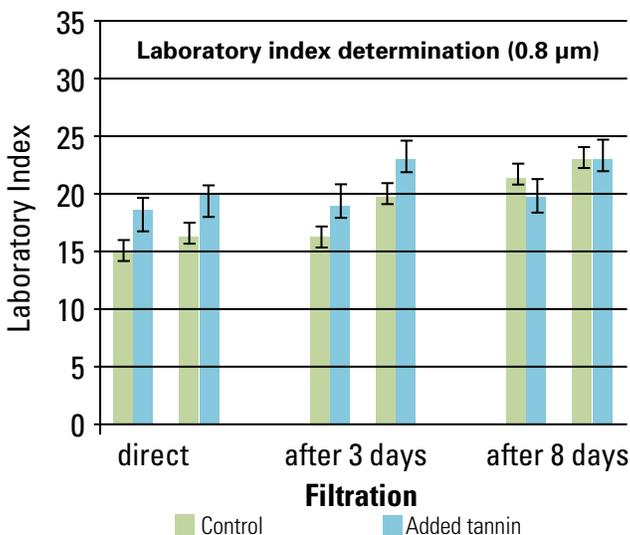
**Fig. 3:** Laboratory index measurement (0.8 µm), control sample compared with immediate tannin addition, after three days, and after eight days (note: error indicator: control: 1.2, tannin addition: 1.5), evaluation: Jelena Bohn
