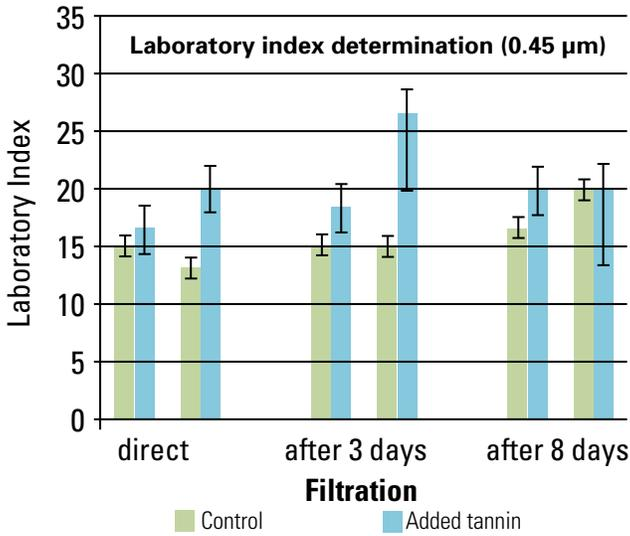
**Fig. 1:** Laboratory index measurement (0.8 µm), control sample compared with immediate tannin addition, after three days, and after eight days (note: error indicator: control: 1.2, tannin addition: 1.5), evaluation: Jelena Bohn
