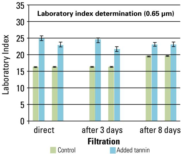
**Fig. 2:** Laboratory index measurement (0.65 µm), control sample compared with immediate tannin addition, after three days, and after eight days (note: error indicator: control: 0.1, tannin addition: 0.7), evaluation: Jelena Bohn
