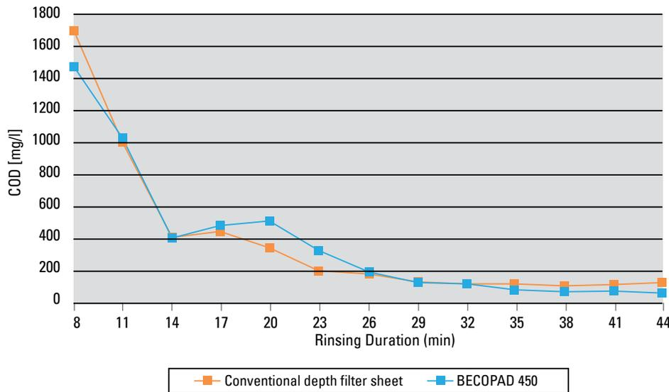
**Figure 1:** Graph of COD value over rinsing duration
