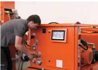
Image 1: Eaton's XV300 HMI-PLC will be used in all future DILO service equipment.
