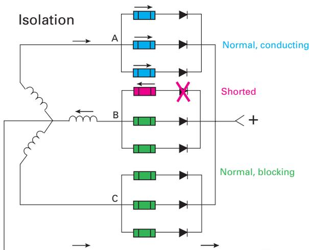
Fuse on shorted diode in leg B should be able to open and clear before any damage is done to the diodes in leg A
