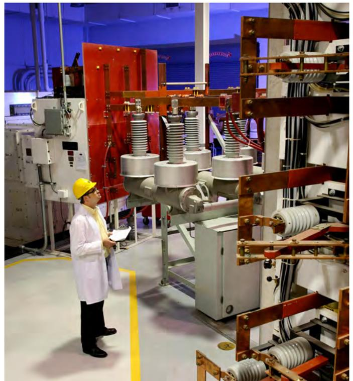
The Eaton Bussmann Division’s Paul P. Gubany Center for High Power Technology is the electrical industry’s most comprehensive facility for testing and certifying device and equipment SCCRs. Capable of performing electrical tests up to 600 V three-phase, 300 kA of short-circuit current for meeting ANCE, ANSI, CE, CSA, ETL, IEC and UL testing requirements.
