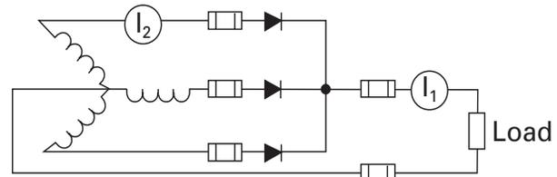
Figure 50: Three-phase, half-wave.
