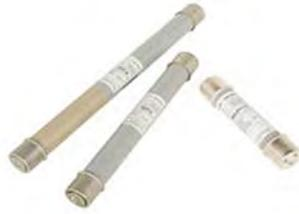
Low amp, E-Rated medium voltage fuses are general purpose current-limiting fuses defined by their melting time-current characteristic that permits their electrical interchangeability with fuses having the same E-rating. To be E-Rated, the fuse responsive element shall melt in 300 seconds at a RMS current within the range of 200% to 240% of the fuse's continuous current rating. (For fuses rated 100E or less)(ANSI C37.46).
