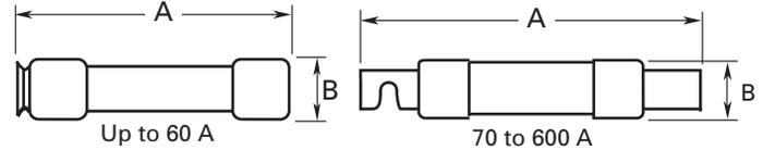
Basic dimensions are same as Class H(K), general purpose (NON and NOS) fuses. **Note:** relating to dimensional compatibility these fuses can replace existing Class H, RK1 and RK5 fuses.
