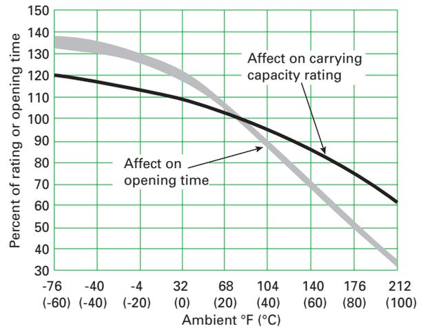
Figure 16: Ambient temperature dual-element fuse derating curve.
