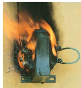
**Figure 18:** Fires can result if the correct OCPD amp rating is not applied.
