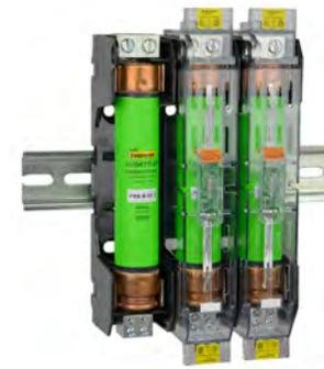
Bussmann series modular Class R fuse blocks feature a snap-together construction to create the required number of poles. Either DIN-Rail or panel mount, these blocks are available with optional covers that provide a lockout/tagout provision for enhanced electrical safety. Also available in power distribution fuse block versions.
