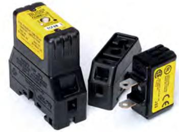
The CUBEFuse mounts in 35mm DIN-Rail and panel mountable amp rating rejecting holders (30, 60 and 100 A) that will not accept a fuse rating greater than the holder's. Additionally, the CUBEFuse can be mounted in the UL 98 Compact Circuit Protector available in 1-, 2- and 3-pole factory configured units in the same 30, 60 and 100 amp rating rejection increments.
