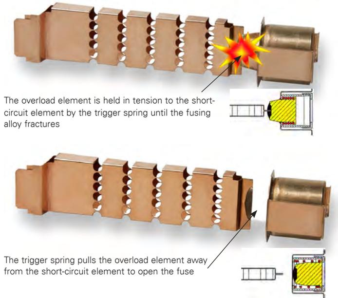
**Figure 10:** Overload element operation.
