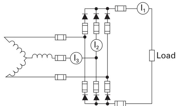
Figure 51: Three-phase, full-wave.
