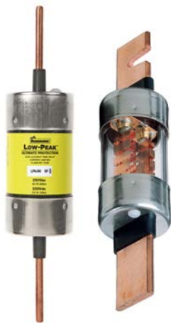
Figure 3.1.1.a A regular and x-ray view of the Bussmann™ series Low-Peak™ LPN-RK dual-element fuse showing the overload and short-circuit links.
