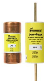
Figure 3.1.6.1.b Low-Peak Class J fuses achieve rejection by their unique physical size that is unlike other UL class fuses.
