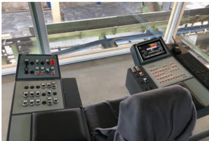
The core of the new system is an XV300 HMI/PLC with integrated touch display, which is built into the control chair in the control room and allows the operator to control all system drives and functions.
